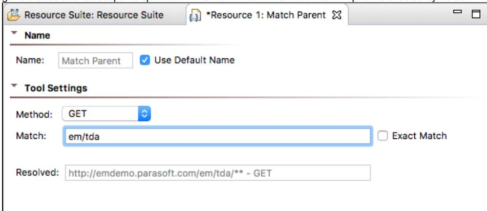
When SOAtest determines a match in the Resource Template, configurations from all chained tools are applied. You can determine how to structure template files and configure matching patterns accordingly. See [Example Smart Test Template](#) for a common use-case.
