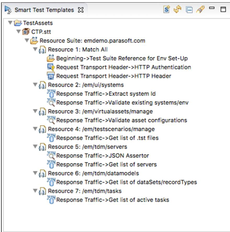
The resource suite is configured to match any scheme, port, and path at host "emdemo." As a result, any tests generated for emdemo will include tools references in the Test Reference Suite. Additionally, tests will be configured with authentication and header settings configured in the HTTP Authentication and HTTP Header tools, respectively.
