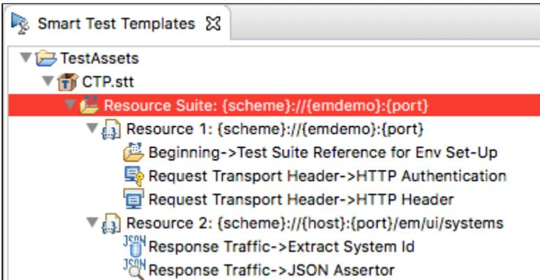
When the SOAtest creates a new smart API test, it will read and apply the rules specified in the .stt file.
