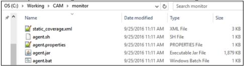
4. Open the %WORKING\_DIR%\monitor folder and run the agent.bat script. A command window will open and display a JVM arg string to add to your Tomcat server startup process:
