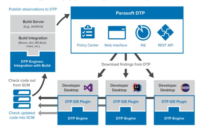
Parasoft Jtest ships with DTP Plugins for Eclipse, IntelliJ IDEA and NetBeans that enable you to integrate Jtest into your IDE. This allows you to leverage the capabilities of the DTP Engine within your development desktop, import findings from DTP into the IDE, as well as utilize additional capabilities available for Jtest Desktop, such as creation of unit testing artifacts.
