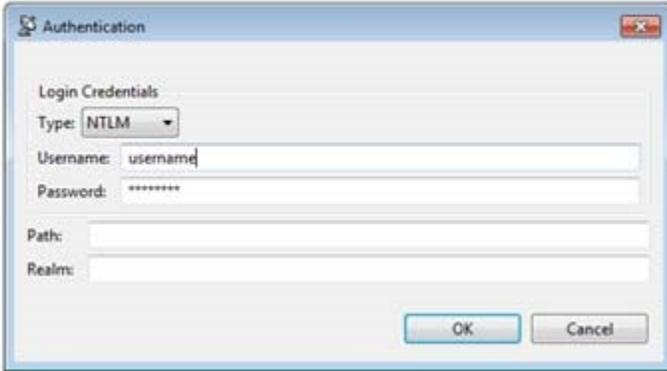
You can enter multiple authentication credentials for scenarios that access many servers which authenticate in different ways. SOAtest will use the path and realm to determine when the authentication scheme should be applied to a request.
