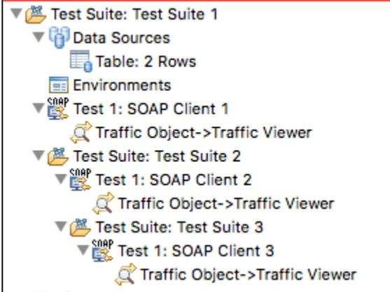
In this case, we assume that **Tests are individually runnable** is enabled for Test Suite 2 and Test Suite 3, the Table has 2 rows of data, and a test is run under each of the Test Relationship options for Test Suite 1. The following table demonstrates the order that tests would run for different choices of Execution Options of Test Suite 1. This also assumes that **Run individually** is enabled for Test Suite 2 and Test Suite 3.
